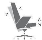
syncro mechanisms and seat inclination adjustment
